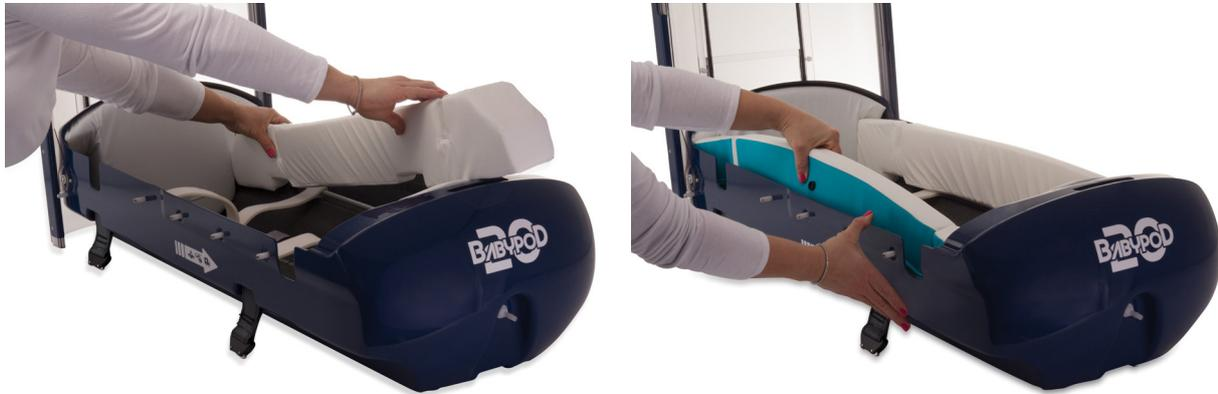
Insert the "Base" foam section into the bottom of the Baby Pod, making sure to keep the 4 Infant Positioning Straps Accessible. On top of this, place Vacuum Mattress with the vacuum port at the Foot end of Baby Pod 20 with the valve facing up. The valve should be in the open position (tubing sections fully engaged with the black "O" ring hidden from view) to allow air to enter the mattress. Spread the polystyrene bead contents of the mattress evenly by hand.
