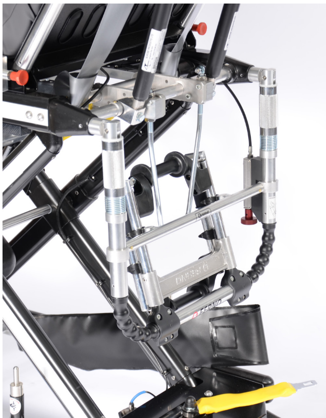
Figure 23 - Ensure push/pull overlaps the U-bolt
