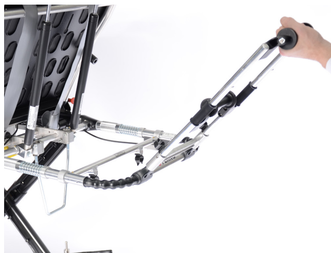
Figure 27 - Push knurled sleeves down over hinge
