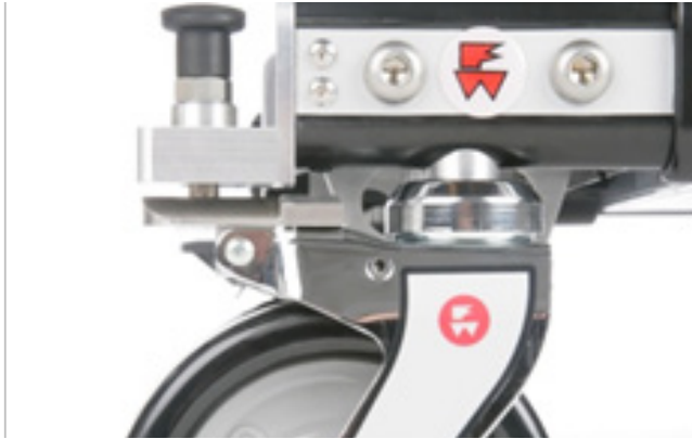
Figure 38 - Position location pin to apply wheel lock
