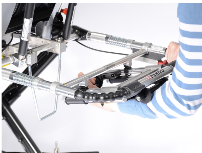
Figure 24 - Release push/pull from clips
