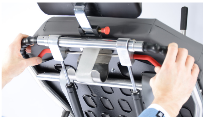
Figure 14 - Press either red lever to raise/lower backrest
